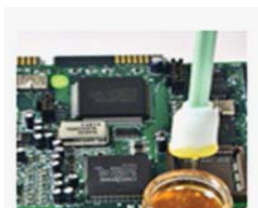
Apply Flux to PCB Chip Leads
