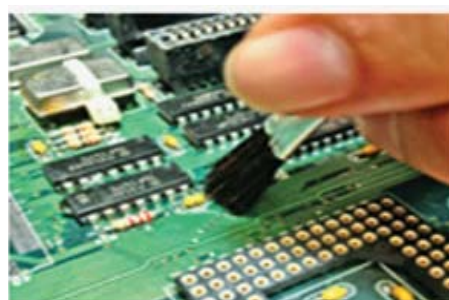
SCRUBBING OLD FLUX AWAY WITH SOLVENT OFF I.C LEADS
