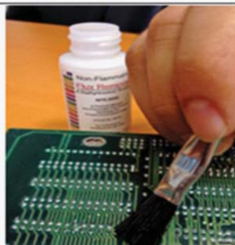
CLEANING PC BOARDS SOLDER JOINTS AFTER REWORK
